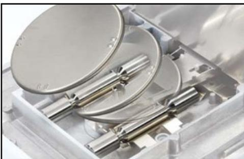
AutoCal™ internal calibration system automatically calibrates the balance when it senses a temperature change significant enough to affect the weighing accuracy.
